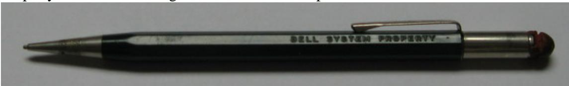
To disassemble the “spiral” pencil, grasp the knurled writing tip in one hand, and the dark green barrel in the other, and gently pull the writing tip straight out of the pencil. The “innards” are held in place simply by friction, and usually come out easily. Be very careful to keep the “innards” in line with (aligned with) the barrel as you pull, so the “spiral” doesn’t get bent.
